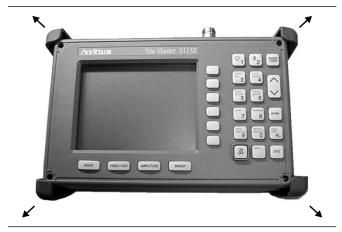
Figure 10. Removing the Corner Bumpers
